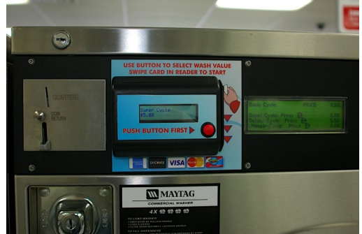
Maytag 40 lb Front Load Washer With Wireless Credit and Debit Card Swipe Installed
